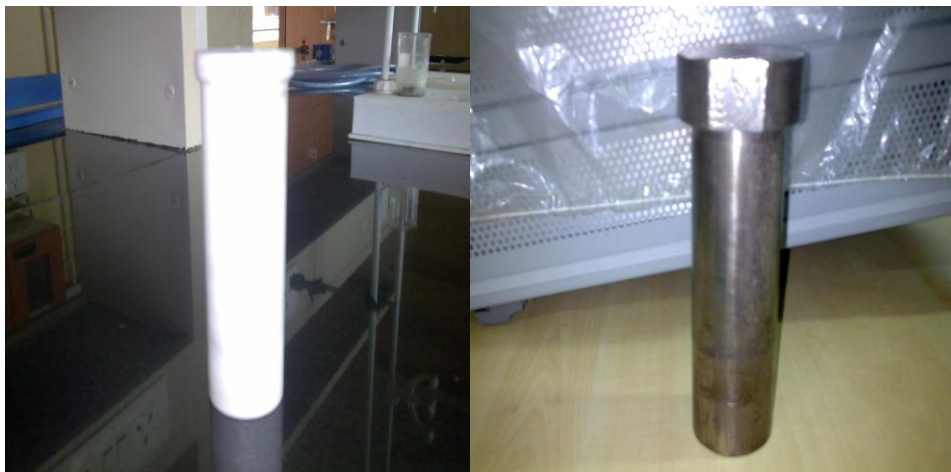
Fig.2.4: The Home fabricated Stainless Steel chamber and the Teflon chamber where all the synthesis were done.
