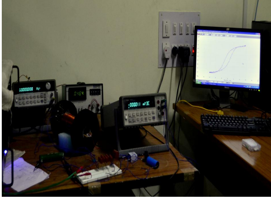
Fig. 2.20: Photograph of the experimental set-up for measuring hysteresis loops.
